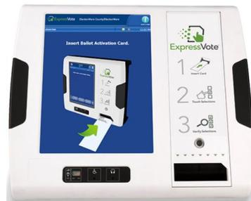
Pictured above is the Ballot Marking Device. A blank ballot is inserted into it, you make your selections, and your voted ballot is printed out. You then place your voted ballot into the ballot box.
